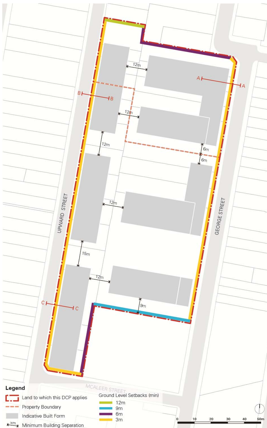
Figure 4 - Building Setbacks and Separation
